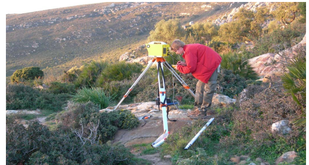
Figure 1. ILRIS 3D TLS in field.
