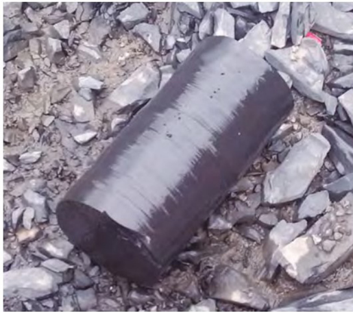
Figure 10. Shale core from Jiao-Shi-Ba, Chongqing province (W. H. Zhang et al., 2016), with obvious layers.
