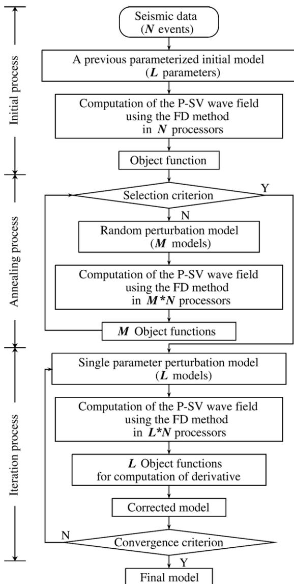
Fig. 6. Flow chart of the proposed sequential waveform method.
