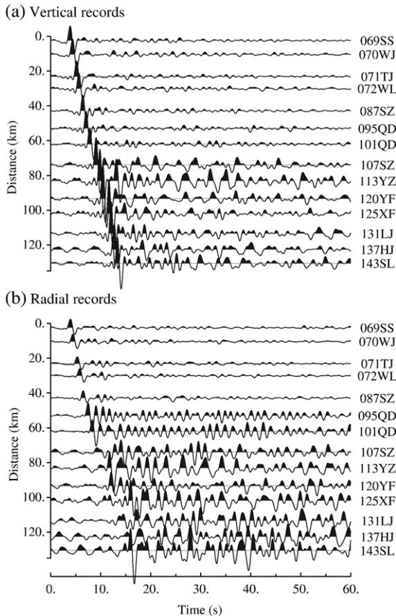
Fig. 8. Observed seismograms generated by event ep04705 (Table 2) and recorded at the stations (labeled on the right of each waveform) belonging to the profile B-B'. The traces represented in the upper part (a) provide the vertical ground motion, while those plotted in the lower part (b) give the radial ground motion. Clear basin effects can be observed.
